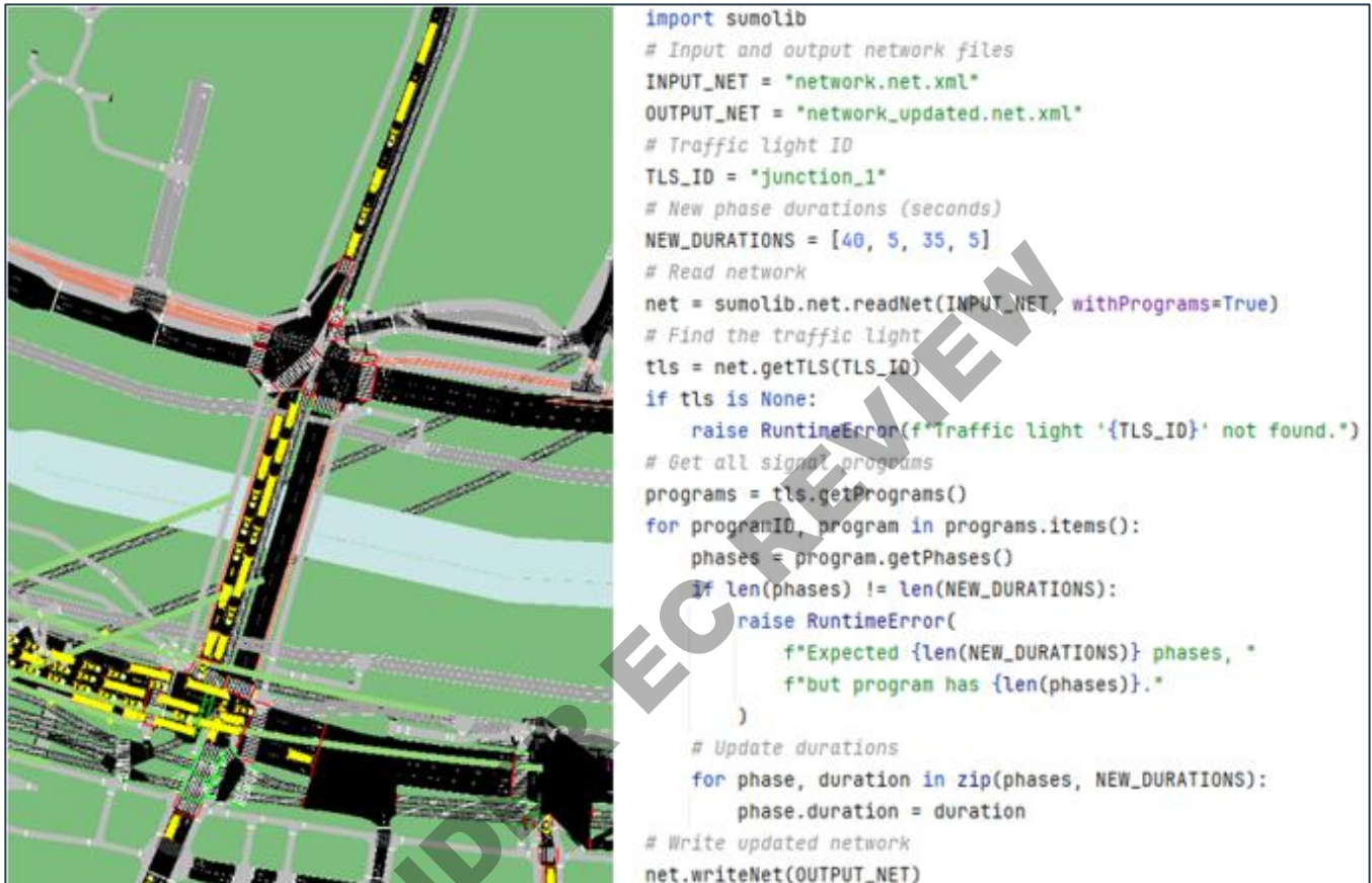
Figure 24: A screenshot for intersections with traffic lights in SUMO and a sample of python script for updating the schedules of a traffic light
